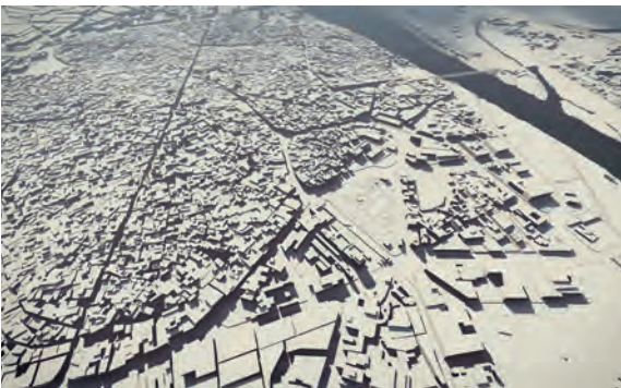
As a background for the interactive map of Mosul, high resolution satellite imagery provided by the DigitalGlobe system was used. The selected image was vectorized into a high detailed topographic map of Mosul and transformed into a 3D model of the historical center of the city (archive of the Oriental Institute, the Czech Academy of Sciences)
