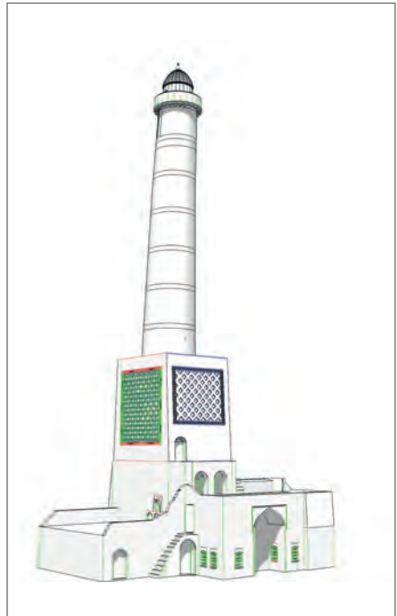
The surface model. Not only the edges of the 3D object, but also its surfaces are defined (archive of the Oriental Institute, the Czech Academy of Sciences)
