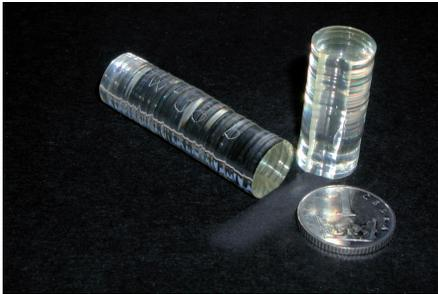
Fig. 7. Scintillation crystal of PWO grown by the Czochralski method in the Institute of Physics, Czech Academy of Sciences
